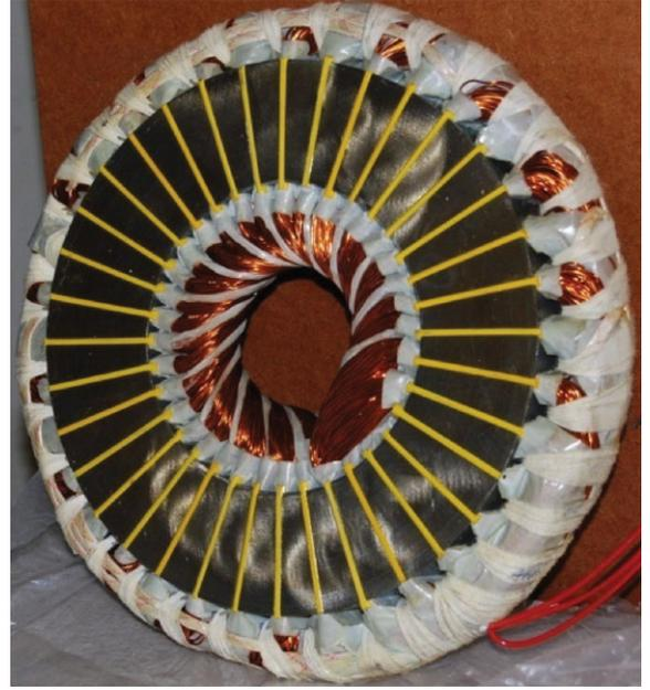
Fig. 4. Axial flux stator used for MGPM machine
