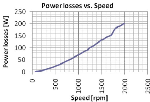
Fig. 12: Experimental results of the no-load test
