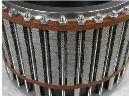
(c) Modulator support rods. Cavities to be filled with epoxy.
