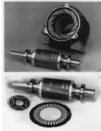
Fig. 1. Normal laminated flux barrier rotor RSM.
