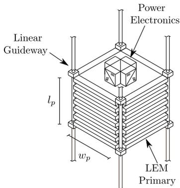
Fig. 1: Example piston in the LEM-GES system, excluding the armature winding.
