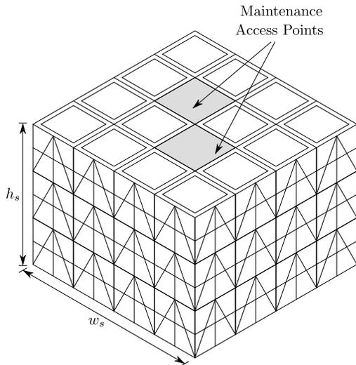
Fig. 3: An outside view of an example 14 shaft LEM-GES structure.
