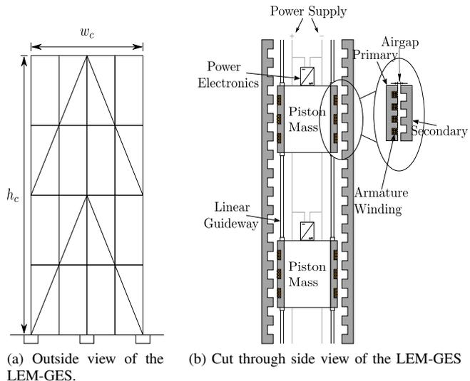
Fig. 2: An outside view and a cut through side view of a single shaft of the proposed LEM-GES system.
