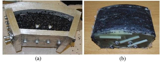
Fig. 18. (a) Dummy stator mould being prepared with plastic pellets and epoxy resin and (b) completed nonmagnetic dummy stator section.
