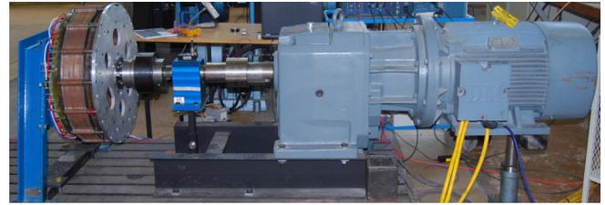
Fig. 13. Prototype toroidal-winding PMSG mounted on the test bench in the laboratory.
