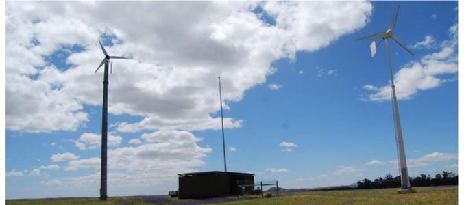
Fig. 10. SS-PMGs 1 and 2 integrated as complete wind turbine systems, being field tested.
