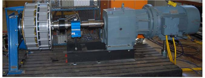
Fig. 9. Prototype 15-kW SS-PMG 2 on the test bench, connected to a driving motor on the right, through a torque sensor shown in the middle.
