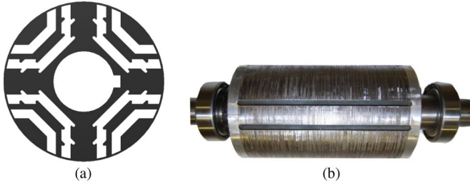
Fig. 9. Constructed unskewed ideal rotor configuration. (a) CAD sketch of proposed RSM rotor laminations. (b) Epoxy-filled unskewed ideal rotor with ribs removed.
