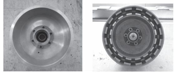
Fig. 5. Prototype loss drum (left) and DSR PM rotor (right).
