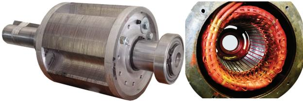
(a) Rotor (b) Stator
