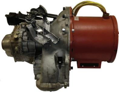
Fig. 17: RS motor together with the 5-speed manual gearbox and differential.
