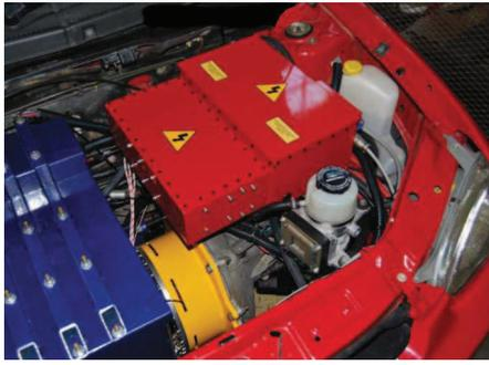
Fig. 2: E-Corsa with traction motor (yellow), inverter (red) and battery pack (blue).
