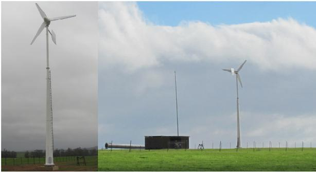
Fig. 9. Field testing of the 15 kW directly grid connected SS-PMG wind turbine system.
