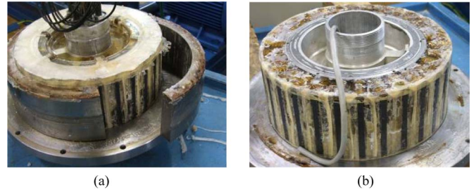
Fig. 9. Prototype 10-kW 40-pole/30-slot stator manufacturing. (a) Removing the stator mold. (b) Finished stator.
