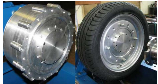
Fig. 10. Prototype 10-kW 40-pole/30-slot concentrated-coil EV PM hub motor with open slots and interior PM rotor.
