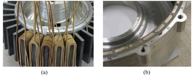
Fig. 8. Prototype 10-kW 40-pole/30-slot stator and PM rotor. (a) Stator laminations and windings. (b) Rotor laminations and magnets.
