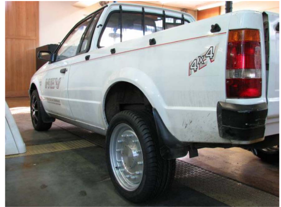
Fig. 17. Prototype 10-kW 40-pole/30-slot in-wheel PM hub motor installed on a small utility vehicle for testing.
