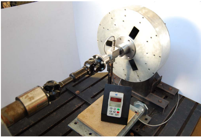
Fig. 10. Wind generator test setup with torque sensor.
