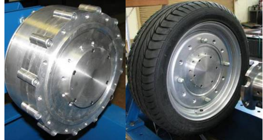
Fig. 8. Prototype 10 kW 40-pole/30-slot concentrated-coil EV in-wheel PM machine with open slots and interior PM rotor.
