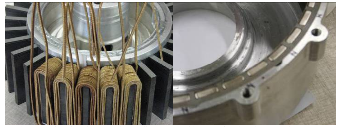
(a) stator laminations and windings (b) rotor laminations and magnets Fig. 7. Prototype 10 kW 40-pole/30-slot machine.
