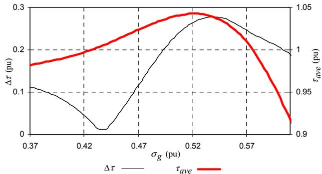
Fig. 4. Per unit cogging torque and average torque versus slot width of the irregular parallel slotted machine (Fig. 1a).
