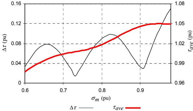
Fig. 2. Per unit cogging torque and average torque versus magnet pitch of the irregular parallel slotted machine (Fig. 1a).
