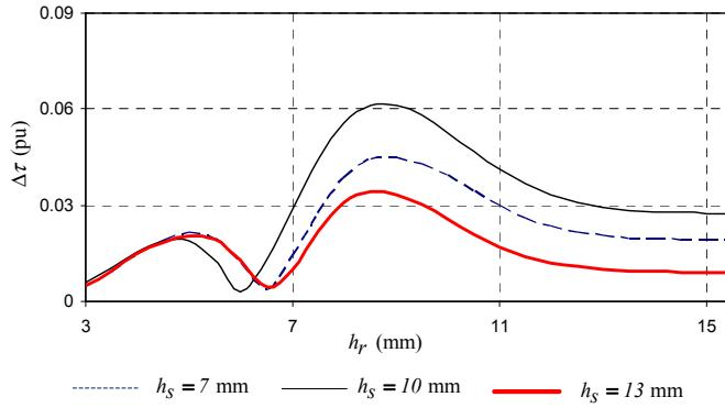
Fig. 10. Per unit cogging torque versus rotor yoke height with stator yoke height a parameter of the irregular parallel slotted machine (Fig. 1a).
