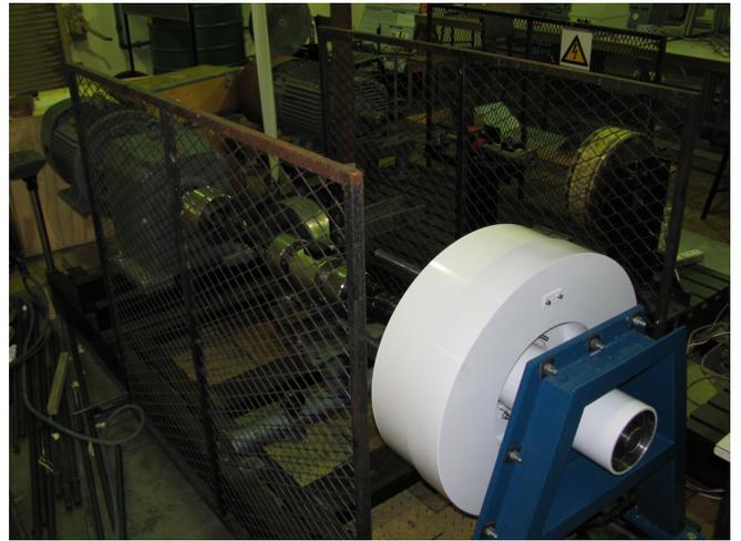
Fig. 13. 15 kW PM wind generator prototype on the test bench.
