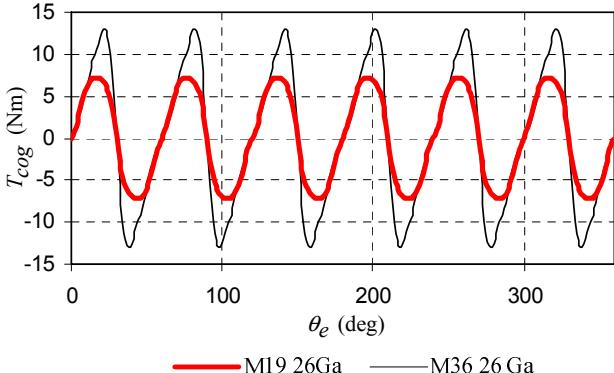
Fig. 12. Cogging torque waveforms of the prototype PM wind generator for two different lamination steels.
