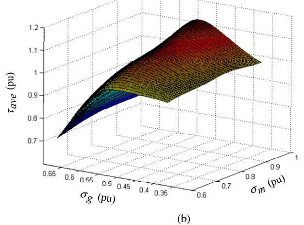
Fig. 5. (a) Per unit cogging torque and (b) average torque versus slot width and magnet pitch for the irregular parallel slotted machine (Fig. 1a).
