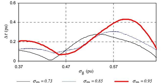
Fig. 8. Per unit cogging torque versus slot width with magnet pitch a parameter of the irregular parallel slotted machine (Fig. 1a).
