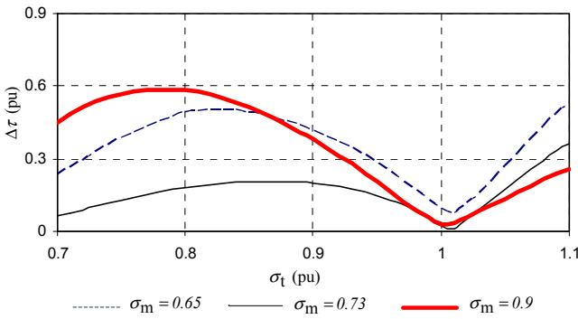
Fig. 9. Per unit cogging torque versus slot pitch with magnet pitch a parameter of the irregular parallel slotted machine (Fig. 1a).
