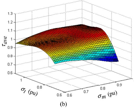
Fig. 6. (a) Per unit cogging torque and (b) average torque versus slot pitch and magnet pitch for the irregular parallel slotted machine (Fig. 1a).
