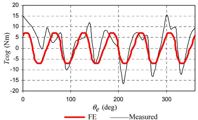
Fig. 15. Measured and FE-calculated cogging torque waveforms of the PM wind generator prototype.
