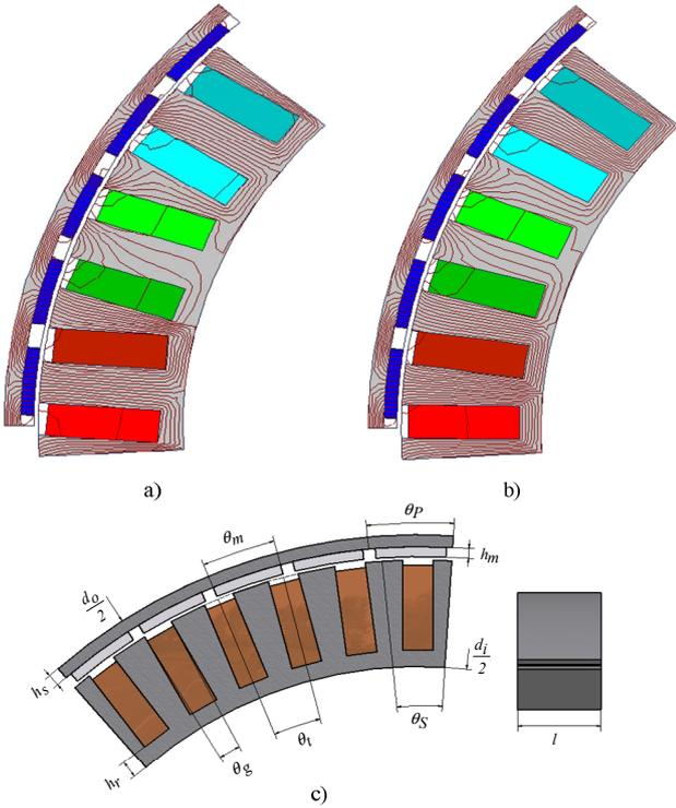
Fig. 1. (a) Irregular parallel slotted, (b) regular taper slotted PM machine sections used in the FE analysis, (c) section view with design parameters.
