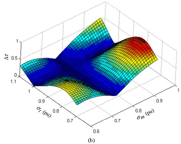
Fig. 7. Per unit cogging torque of the regular taper slotted machine (Fig. 1b) versus (a) slot width and magnet pitch; (b) slot pitch and magnet pitch
