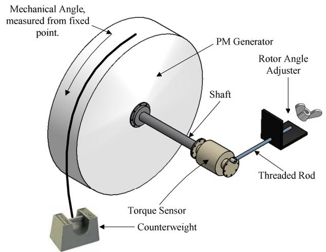
Fig. 14. Static cogging torque measurement by changing the rotor angle in discrete steps and taking the static torque reading at each rotor-angle step.
