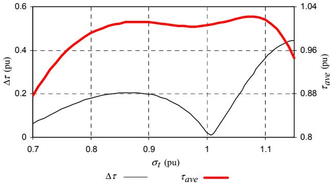
Fig. 3. Per unit cogging torque and average torque versus slot pitch of the irregular parallel slotted machine (Fig. 1a).
