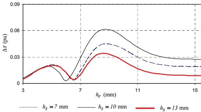
Fig. 10. Per unit cogging torque versus rotor yoke height with stator yoke height a parameter of the irregular parallel slotted machine (Fig. 1a).
