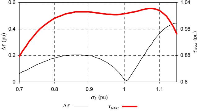
Fig. 3. Per unit cogging torque and average torque versus slot pitch of the irregular parallel slotted machine (Fig. 1a).
