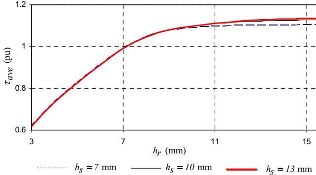
Fig. 11. Per unit average torque versus rotor yoke height with stator yoke height a parameter of the irregular parallel slotted machine (Fig. 1a).
