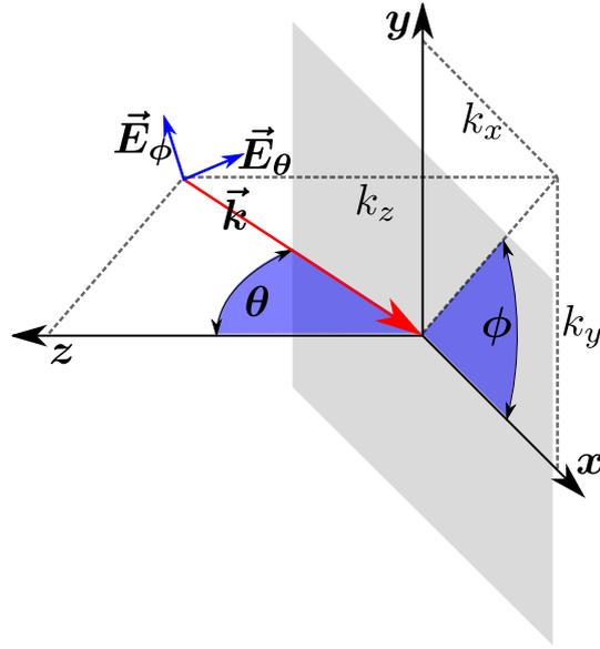
Fig. 1. A diagram showing an incident plane wave with arbitrary linear polarisation and direction of incidence ( $\vec{k}$ ). The definitions of the angles (blue arcs) used in the calculation of the radar cross section of an object located at the origin and the square PEC plate (grey) considered in this paper are also shown.
