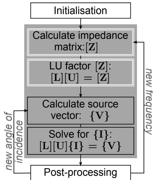
Fig. 2. A block diagram showing the steps involved in obtaining the method of moments solution for a typical scattering problem. The phases considered here for timing purposes are surrounded by a grey box and the phases for which GPU acceleration is applied also highlighted by double white outlines.
