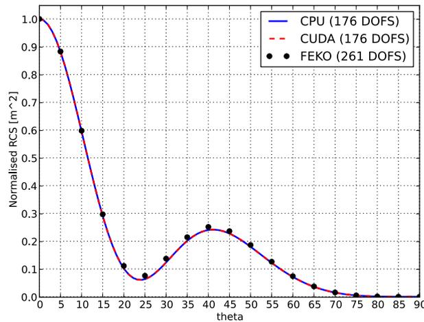
Fig. 9. The computed normalised radar cross section of the square plate shown in Figures 7 and 1 as a function of angle  $\theta$  ( $\phi = 0$ ). Results computed using FEKO as well as the CPU and CUDA implementations discussed here are shown.
