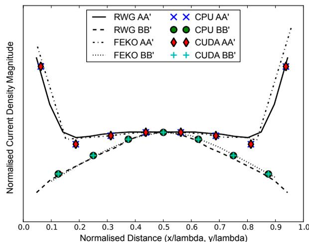
Fig. 8. A recreation of Figure 6 from [14] showing the normalised current density magnitude along the two cut lines in Figure 7. Results from [14] along with results computed using FEKO and the two implementations discussed here are presented.
