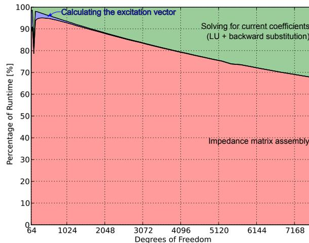
Fig. 10. The relative contribution of the three timed phases in the solution process as a function of the number of degrees of freedom in the mesh. The problem shown in Figure 7 is solved using the CPU implementation.
