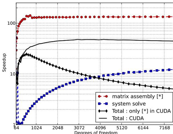
Fig. 13. The measured speedup of the matrix assembly (●) and solution of the linear system (■) as a function of the number of degrees of freedom. The combined speedup (—) as well as the speedup when only the matrix assembly phase is accelerated (◆) is also shown. A logarithmic scale is used on the vertical axis for better comparison.
