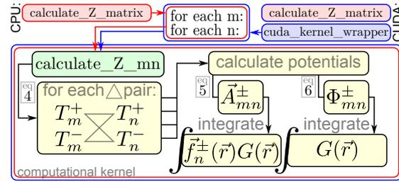
Fig. 5. A block diagram showing the computational process of the method of moment matrix assembly phase for both the CPU and CUDA implementations. The execution path for the CPU implementation is shown in red, with the GPU execution path shown in blue. Common elements are outlined in black and make up the shared computational kernel. The relevant equations from Section II-B1 for various sections are also indicated.
