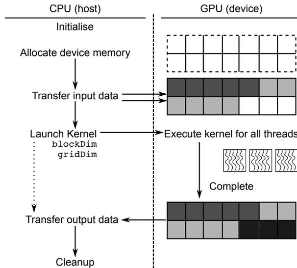
Fig. 4. A diagram showing the program flow of a typical CUDA application. `blockDim` and `gridDim` represent the dimensions of each block and the grid and are used for kernel execution.
