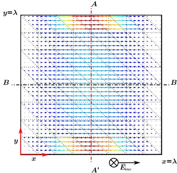
Fig. 7. A figure showing the  $1\lambda$  square plate (lying in the  $xy$ -plane) used as a sample problem in this paper. The mesh (with 176 degrees of freedom) used to obtain the verification results as well as the cut-lines and incident field as defined in [14] are also shown. The surface current calculated using the CPU implementation is overlaid as a quiver plot.
