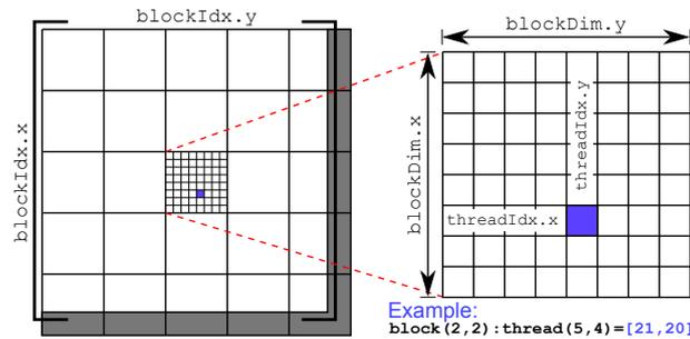
Fig. 6. A diagram depicting the arrangement of threads into two dimensional blocks and blocks into a two dimensional grid as used in this paper. Also shown are the CUDA variables used to determine the identity of a thread at runtime as well as an example thread with global index [21, 20] highlighted in blue.
