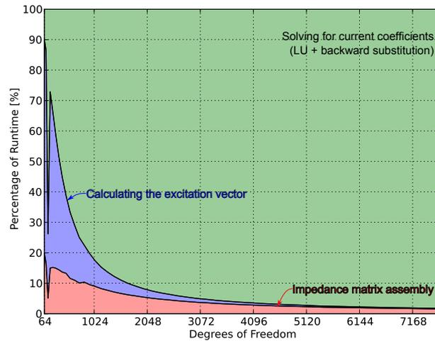
Fig. 11. The relative contribution of the three timed phases in the solution process as a function of the number of degrees of freedom in the mesh. The problem shown in Figure 7 is solved using a CPU implementation with the only matrix assembly phase performed using CUDA.
