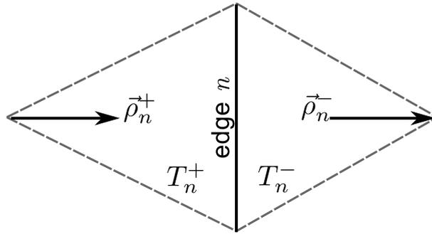
Fig. 3. A diagram of a free edge in a surface mesh as well as the designation of the positive and negative triangles. Also shown are the vectors used in the definition of the basis function associated with the edge.
