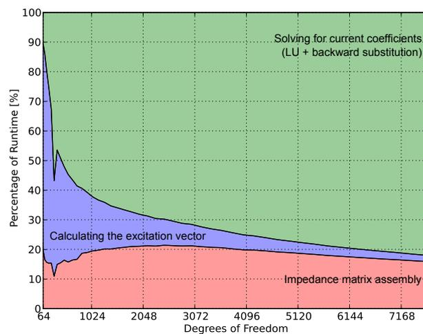
Fig. 12. The relative contribution of the three timed phases in the solution process as a function of the number of degrees of freedom in the mesh. The problem shown in Figure 7 is solved using the CUDA implementation.
